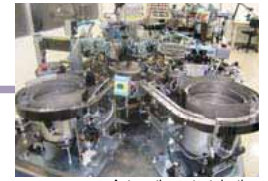
Automatic contact riveting
