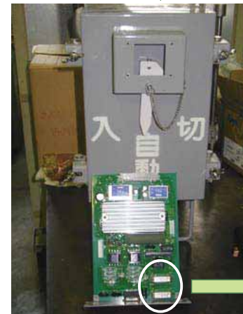
PCB mounted RI-D24T2 type relays for the reply function in the monitoring system
