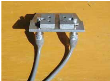
Switch incorporating Bestact that can confirm ON / OFF status
